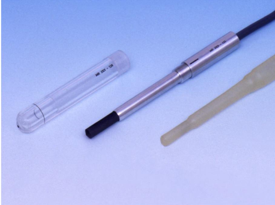
The ionization chamber **MR 2101** exactly corresponds with the construction of its sensitive volume to the widespread design of the chamber NE 2571, developed by Prof. F.T.Farmer.
